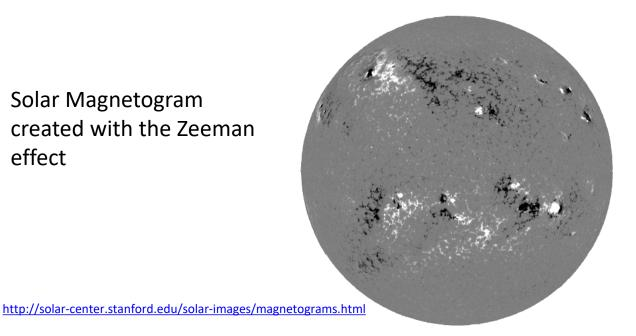
The direction of magnetic field is revealed by the circular polarization of the light
